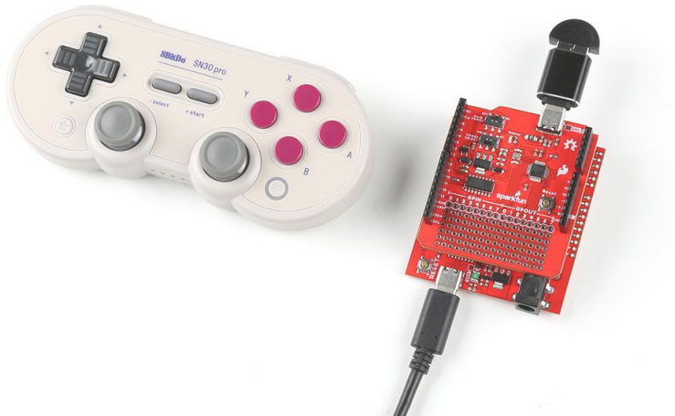
Bluetooth module connected to the USB-C Host Shield; and paired with an 8BitDo controller.
