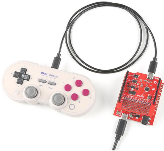
8BitDo controller connected to the USB-C Host Shield with a USB-C cable.
