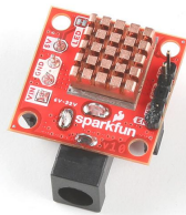
Heat sink attached to the 5V Buck Regulator (AP63357DV).
