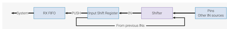
Figure 46. Input Shift Register (ISR). Data enters 1...32 bits at a time, and current contents is shifted left or right to make room. Once full, contents is written to the RX FIFO.
