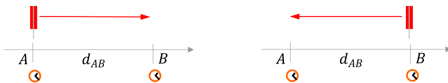
Figure 36: The effect on relative timing of uncertainty in the base station location. This uncertainty is mitigated by using the Timing Advance information from the serving cell.
