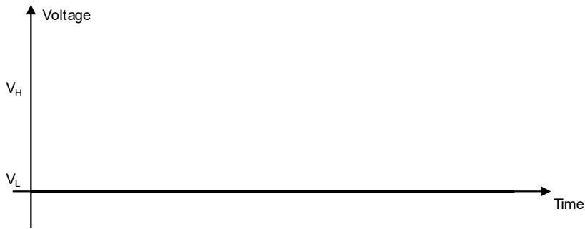
Figure 1: GPIO pin progress for no service
