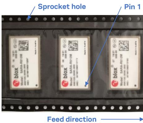
Figure 9: Orientation of SARA-R5 series modules on tape
