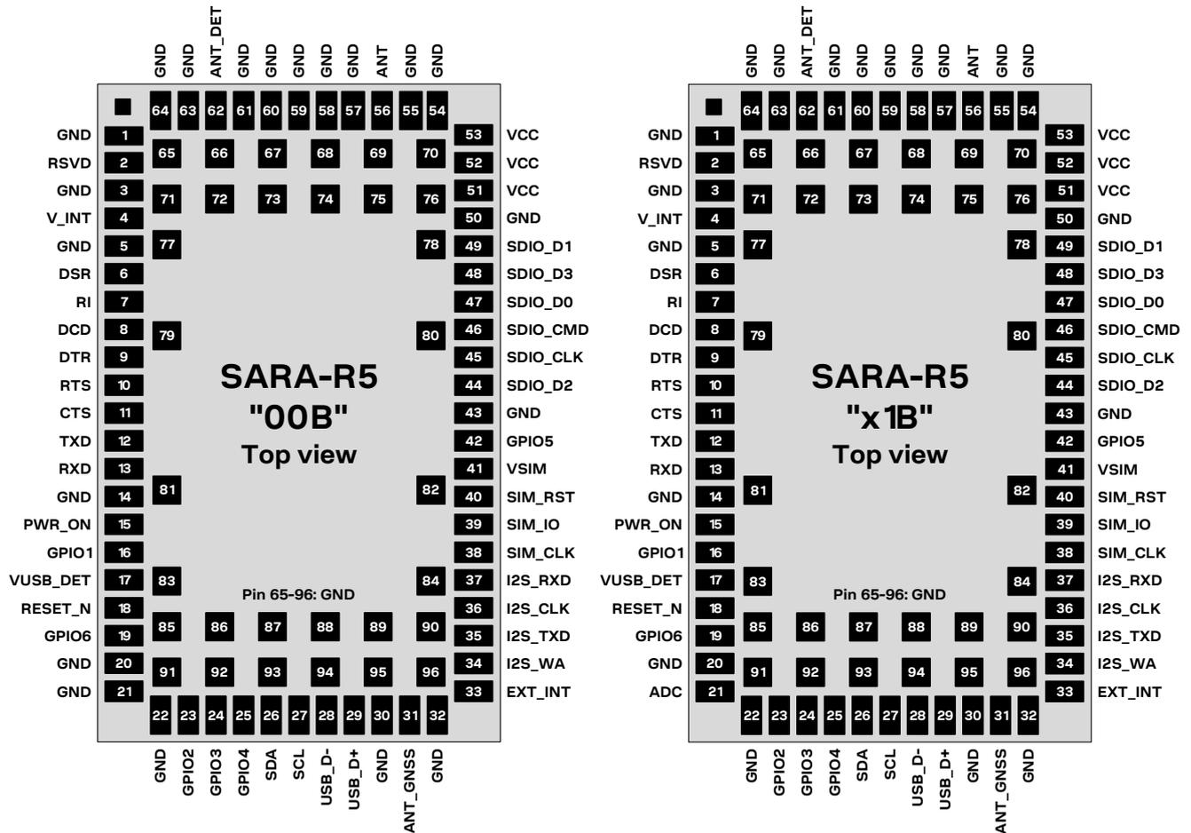
Figure 5: SARA-R5 series modules pin assignment (top view)
