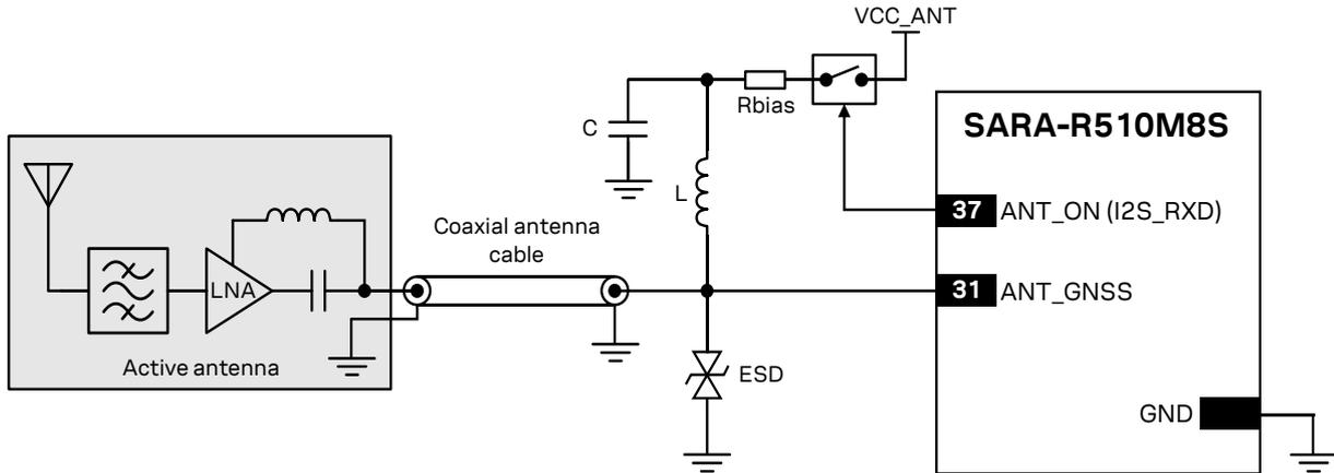
**Figure 45:** Typical circuit with active antenna connected to GNSS RF interface of SARA-R510M8S, using an external supply
