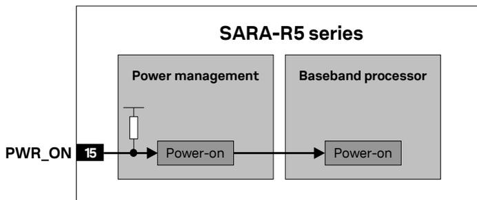
Figure 12: SARA-R5 series PWR\_ON input equivalent circuit description
