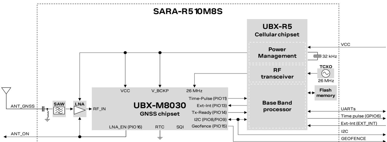
Figure 5: SARA-R510M8S modules GNSS section block diagram
