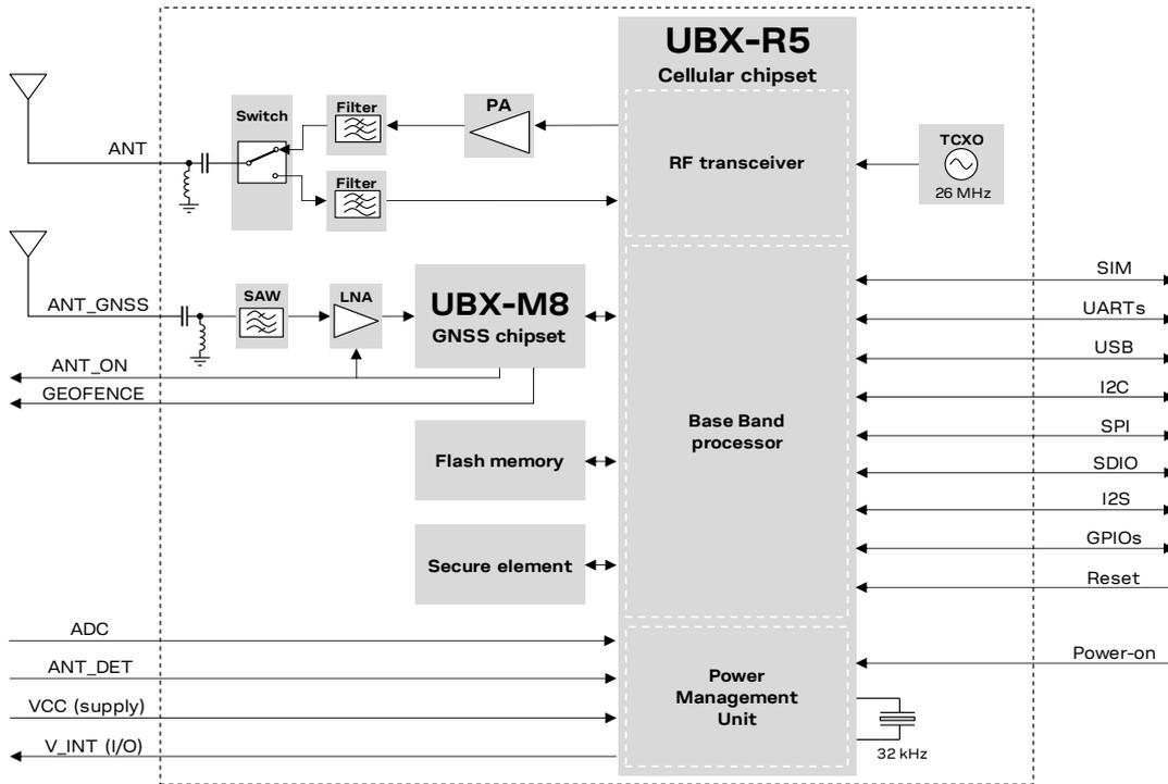
Figure 4: SARA-R510M8S block diagram <sup>2</sup>
