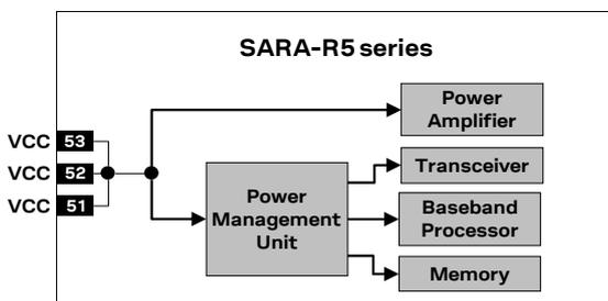
**Figure 7:** SARA-R5 series modules' internal VCC supply routing
