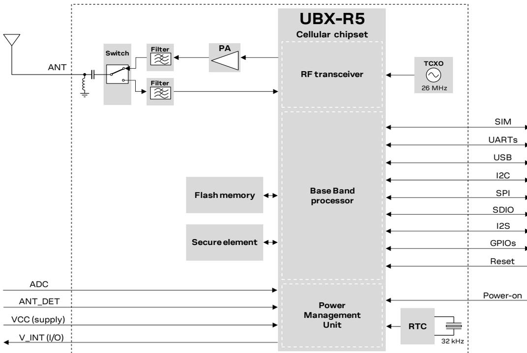
Figure 3: SARA-R510S and SARA-R510AWS block diagram <sup>2</sup>
