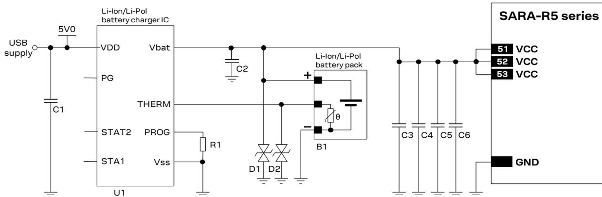
Figure 25: Li-Ion (or Li-Pol) battery charging application circuit
