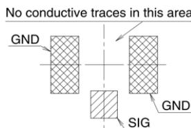
**Figure 37: U.FL surface mounted connector mounting pattern layout**
