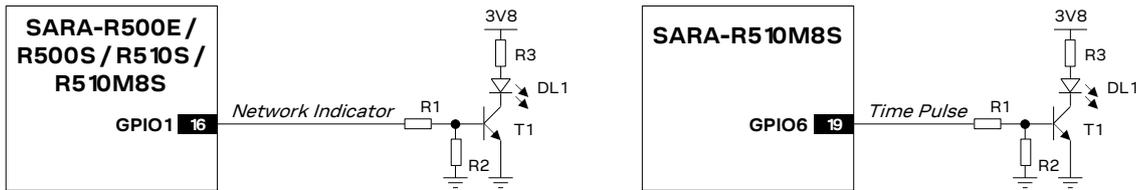
**Figure 71: Application circuit for network indication provided over GPIO1**
