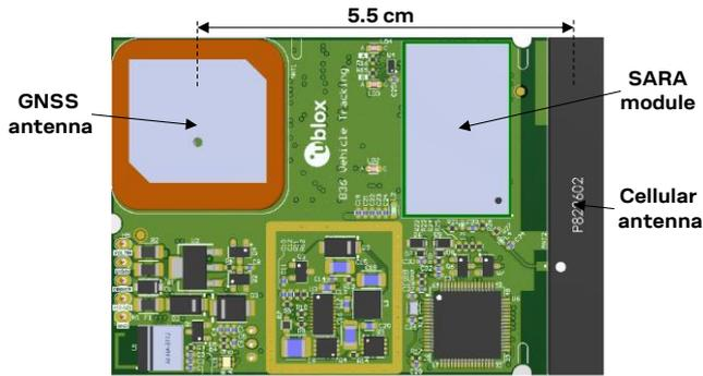
Figure 48: PCB top rendering for the u-blox B36 blueprint with annotated distance between cellular and GNSS antennas
