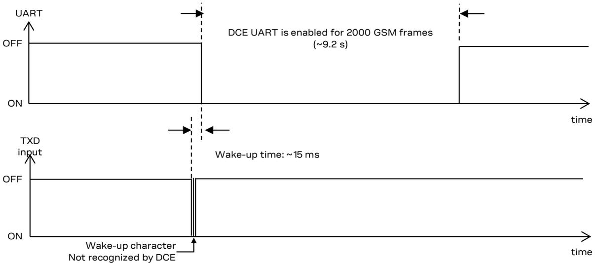
**Figure 20: Wake-up via data reception without further communication**
