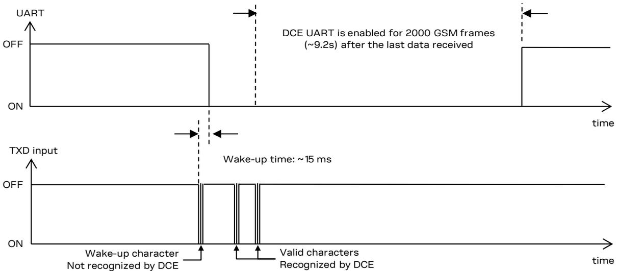
**Figure 21: Wake-up via data reception with further communication**
