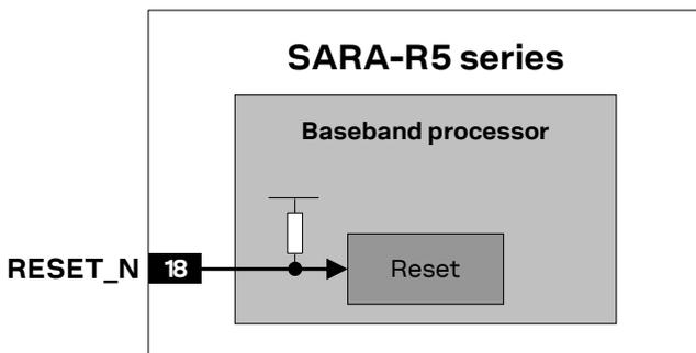
Figure 17: SARA-R5 series RESET\_N input equivalent circuit description
