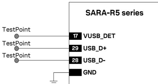
**Figure 67:** SARA-R5 series modules USB application circuit providing access for diagnostic purposes
