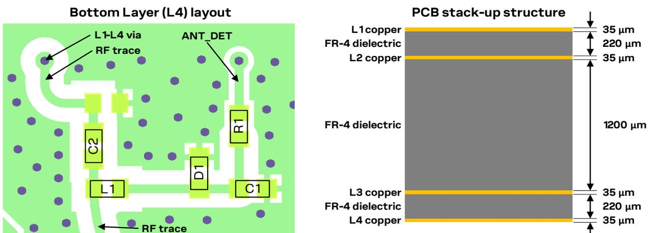
Figure 40: Bottom layer layout and stack-up structure of the u-blox host PCB for the antenna detection circuit
