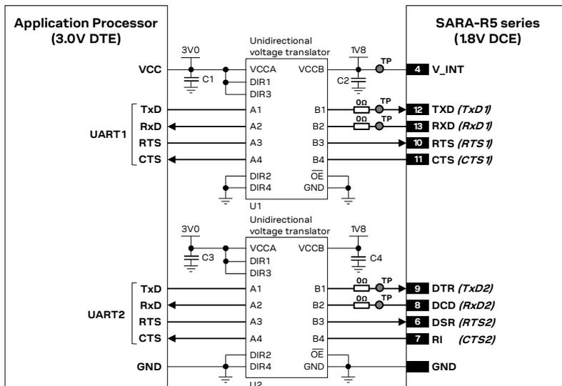
**Figure 62: 2 UART interfaces application circuit with 5-wire links in DTE/DCE serial communications (3.0 V DTE)**
