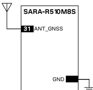
Figure 43: Minimum circuit with GNSS passive antenna
