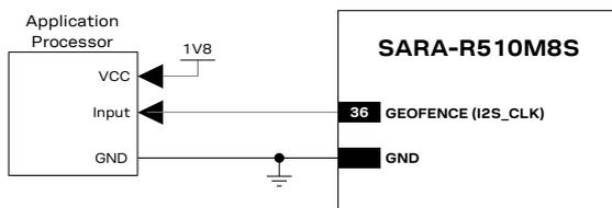
**Figure 72: Application circuit for GNSS peripheral GEOFENCE output pin**
