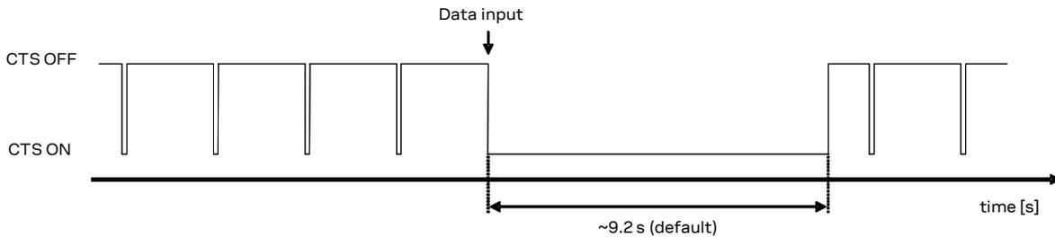
**Figure 19: CTS behavior with power saving enabled (AT+UPSV=1) and HW flow control enabled:**
