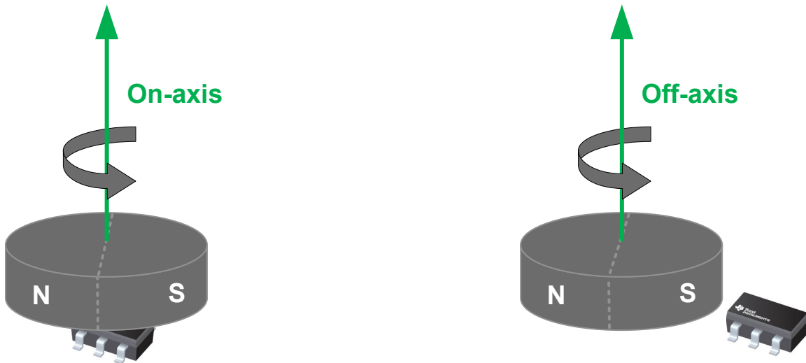
Figure 8-16. On-Axis vs. Off-Axis Angle Measurements
