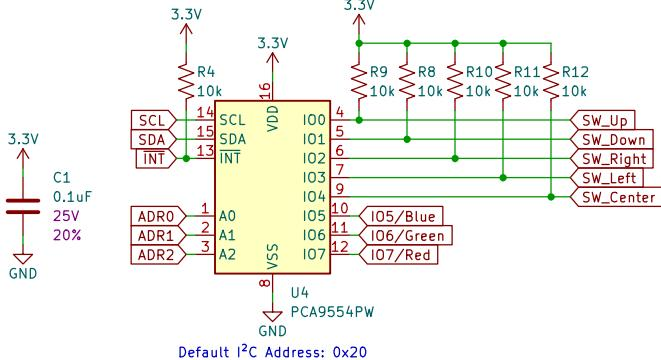
The PCA9554 is identical to the PCA9534 except for the addition of the internal I/O pull-up resistors, which prevents the ports from floating when configured as inputs. Pull-ups are still used in this design so that the '34 can be used if needed.
