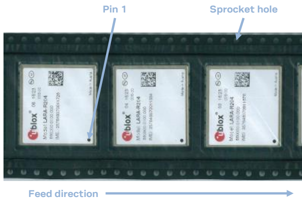
Figure 7: Orientation for LARA modules on tape
