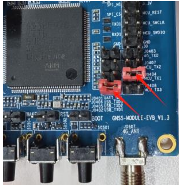
Figure 17: J0402 and J0404 Short-circuited
