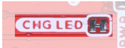
Traces around the CHG LED jumper. (Click to enlarge)
