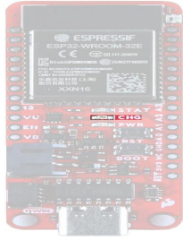
The battery charging ( CHG ) LED indicator on the ESP32-WROOM Thing Plus. (Click to enlarge)
