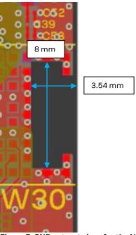
Figure 7: GND cut-out sizes for the NORA-W3x6 PCB trace antenna
