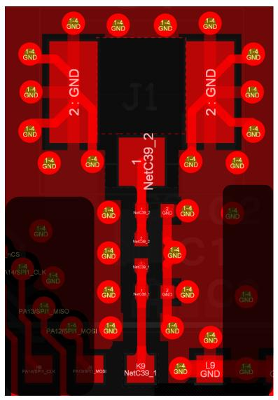
Figure 20: Layer 1 routing, keep-out, and ground stitching vias
