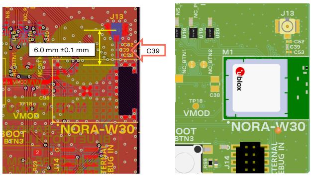
Figure 4: NORA-W301 approved U.FL antenna connection - 2D and 3D views
