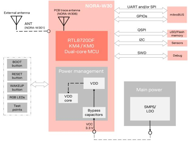
Figure 1: Example of NORA-W30 integrated as a host
