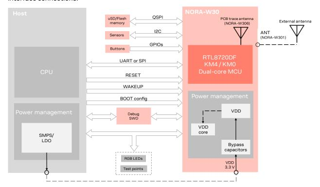
Figure 2: Example of NORA-W30 integration in a host system with external CPU
