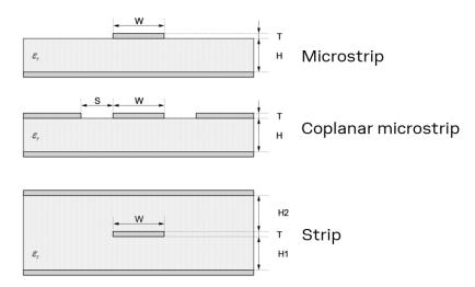
Figure 3: Transmission line trace design
