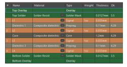
Figure 5: NORA-W301 host board approved layer stack-up
