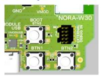
Figure 9: BOOT (BTN3) button to enter the bootloader
