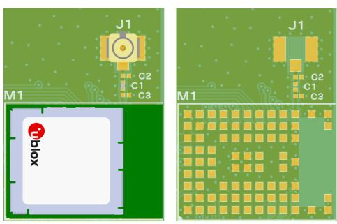
Figure 16: U.FL connector placement (left) and module footprint (right)
