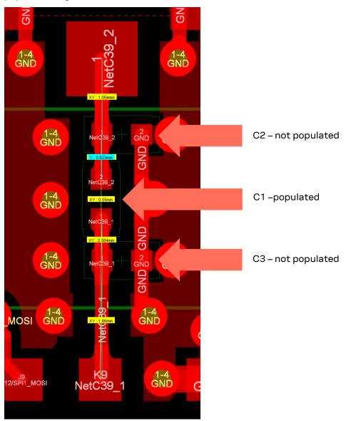
Figure 22: RF trace design component placement
