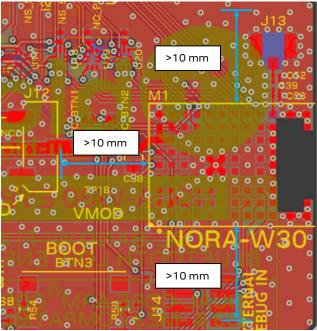
Figure 6: GND plane guard area enclosing NORA-W3x6
