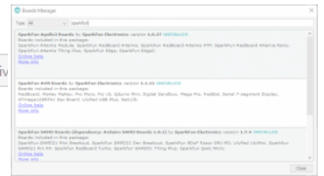
INSTALLING BOARD DEFINITIONS IN THE ARDUINO IDE
